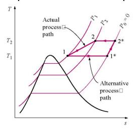
The path is composed of an isothermal process at  $T_1$  from  $P_1$  to  $P_0$  ( $P_0$  is low enough pressure that the gas is an ideal gas or can be taken to be zero), a constant pressure process at  $P_0$  from  $T_1$  to  $T_2$ , and finally an isothermal process at  $T_2$  from  $P_0$  to  $P_2$ . Using the superscript asterisk (\*) to denote the ideal-gas state, the enthalpy change for the real gas is expressed as
